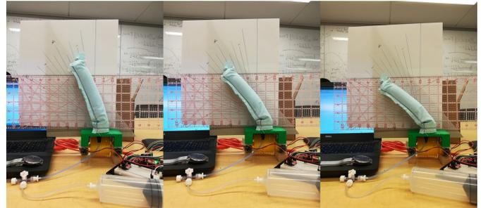
Fig. 5. Characterization setup. The actuator is tested at various lengths and curvature in order to gather data to create a mathematical model of its pathway.
