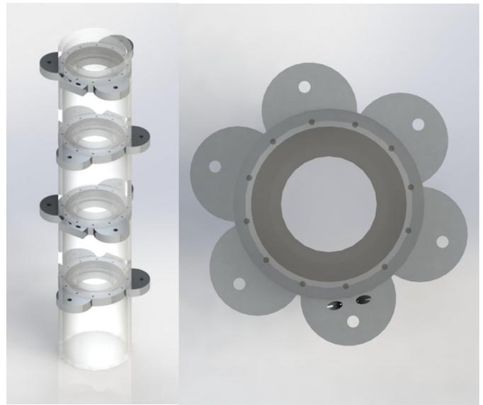
Fig. 1. Acrylic cable guiding plates embedded in silicon finger. The silicon finger has a single pneumatic channel in the middle while the guiding cables are fixed at the end plate and strung through the rest of the plates. The plate has three linear constraint holes for directional constraints and two diagonal constraint holes for roll constraints.
