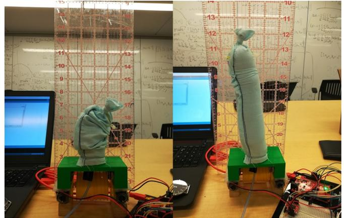
Fig. 4. Volume change of the actuator. The initial length of the actuator is 3 inches. The full length of the actuator is 8 inches.
