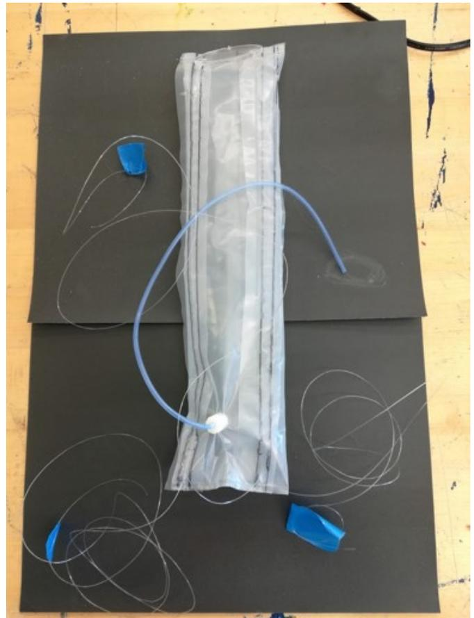
Fig. 2. Hermetic plastic sheet pouch with guiding cables. The channels for the cables are also heat-sealed onto the sheet before creating the finger.
